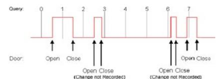
Another example of an application for the State101A is the monitoring of a furnace or pump turning on and off, both of which have a long enough state change to be captured by the State101A.
