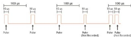
A common application for the Pulse101A is to measure the flow rate or total volume of a pipeline. The Pulse101A collects pulses generated by a flow meter and uses that information to calculate the number of gallons per minute. The flow meter produces a pulse that is too rapid to be collected by the Event101A or State101A, yet can easily be binned by the Pulse101A. The important data here is not the exact time when the pulse took place, but rather the number or pulses in a time interval.
