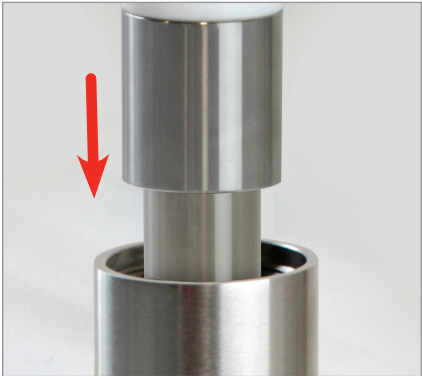
4. Slide the data logger and lid back into the barrier body and screw the lid back on tightly.
