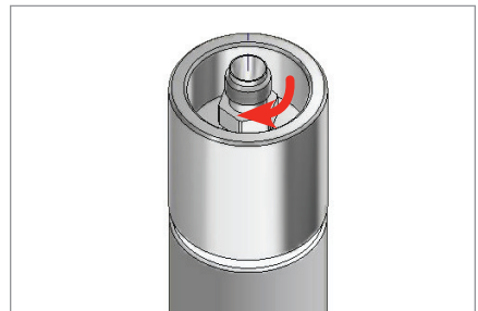
2. Screw the Fitting Body into the end of the stopper assembly (finger-tight).
