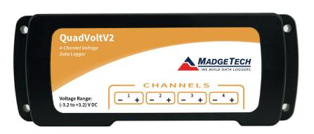
The QuadVoltV2 is an 4-channel, battery powered, DC voltage data logger with a reading rate of up to 4 Hz. It can measure and record 87,296 readings per channel. To maximize memory capacity, users can enable or disable channels. For easy identification, each channel can be named with up to a ten digit title.
