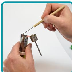
**5** Change the O-Ring seal. Use the O-Ring removal tool to poke into the O-Ring and remove it from the groove. You want to get the sharp end in as tightly as you can, then push down, and then push it to the side so it lifts up and out of the groove. Then use the tool to pull the O-Ring out completely. *Please note that any time you open the MPRF, you must replace the O-Ring with a new one.*
