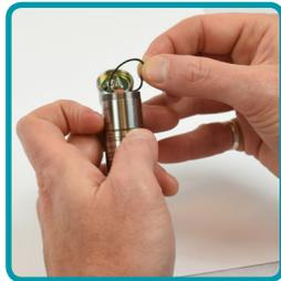
**9** Carefully slide the greased O-Ring over the housing. When it gets near the bottom, you will need to slightly stretch it to get it over the lip on the housing. Carefully push it into the groove. You should not need a lot of force, and rolling your finger around on the O-Ring will help if needed.
