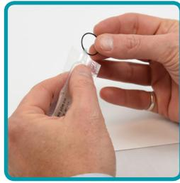
**7** Prepare the replacement O-Ring. Get a little bit of the grease from the o-ring removal tool kit and put some on your fingers. You will only need a small amount. We recommend rubbing the grease between your middle finger and thumb, and then slowly pulling the O-Ring through your fingers to allow the grease to completely cover it. It helps to have a paper towel nearby to wipe your hands once you are done.
