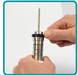
**10** Seal the logger. Use the lock ring and gripper tool to carefully slide it over the probe to get it into place. Hold it loosely and begin screwing the lock ring down first. Once the lock ring is done, you can put some compression on the upper and lower housing and use the gripper tool or Locking Ring Wrench to tighten it. Remove the gripper tool from the logger and you have successfully changed the MPRF battery.
