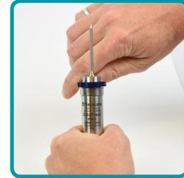
**2** Lift the Locking Ring away. Carefully slide it over the temperature probe and set it to the side. *Note: This Locking Ring could easily become damaged as it is very sensitive to shock dropping on a hard surface.*
