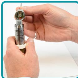
**3** Open up the housing. You'll notice that this lifts away. Try not to pull it too far back because there is a ribbon cable here that can become damaged. The board could also become loose if it gets pulled too hard.
