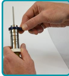
**1** Start by holding the MPRF and squeezing to compress it. Then, loosen up and unscrew the lock ring. Use the gripper tool or the Locking Ring Wrench if this is too tight.
