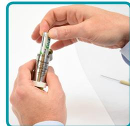
**4** Remove the battery. If it is not sticking out for you to easily grab and pull, it may be stuck. Try giving it a shake and it should come loose. **Make sure to discard of the Lithium battery properly.**
