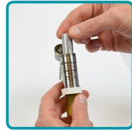
**8** Insert the replacement battery with the positive end down. If you need to know which way to put the battery, there is a marking on the housing of the MPRF that shows the direction it should go.
