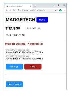
When an alarm is triggered, the remote user can clear and dismiss the alarm.
