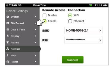
Once the Titan S8 device has been restarted, go to **Settings > Network**, select the Remote Access **Enable** checkbox and select **Connect** to turn back on wireless connection in order to connect to the VNC Viewer.
