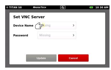
Select the **Device Name** text field to set the Device Name.
