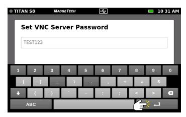
Press in the text box to bring up the virtual keyboard. Some keys are disabled as those characters are not permitted in the Password. Select the Up/Down (Shift) arrow to access additional special characters. The VNC Server Password must be over five characters. Select **Enter** key when finished entering the Password.
