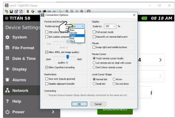
If the Titan S8 screen is distorted when displayed by TightVNC, change the encoding options in the Preferences to **Hextile** which seems to work best for TightVNC.
