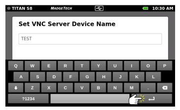
Press in the text box to bring up the virtual keyboard. The space bar is disabled as spaces are not permitted in the Device Name. The Device Name is case sensitive. Select **Enter** key when finished entering the Device Name.
