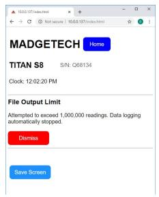
There are other Titan S8 warnings that the remote user can dismiss. There will be a slight delay before the remote user is allowed to dismiss the warning, so the local user has a chance to see the same warning.
