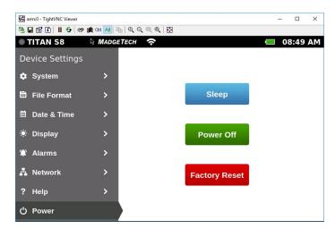
The remote VNC Viewer user now has complete control over the device, including turning off the device and performing a factory reset. **Note:** If the remote VNC Viewer powers off the Titan S8 device, the device must be manually turned back on.
