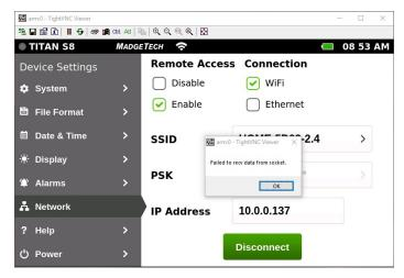
The remote user cannot change the VNC Server password because Remote Access has to be disabled. Disabling Remote Access breaks the VNC Server to VNC Viewer connection.
