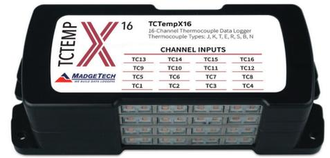
The new TCTempX Series consists of 4, 8, 12 and 16-channel thermocouple data loggers with a reading rate of up to 4 Hz. Improvements include the elimination of an interface cable (uses standard USB-A to Micro USB), increased memory for more readings and increased download speed.
