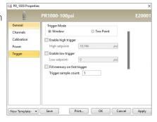
point allows for different Start and Stop setpoints to be defined for both the high and low triggers.
