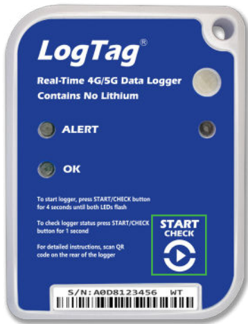
Figure 1: Hold the Start/Check button.
