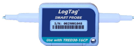
Figure 5: CP110 Smart Probe for TRED30-16CP Loggers
